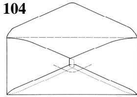
Middle West Envelope Co Knife, rough edges, made with Smithe rotary machine.
