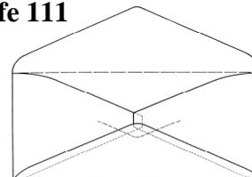
Middle West Knife, rough edges usual; with square side flap ends (15 mm); made with Smithe rotary machine. 105 x 241 mm.
