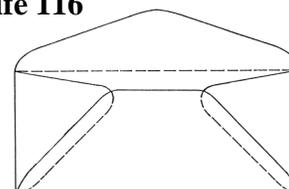
International Envelope Co. Knife, used for all size 23 envelopes from 1950 to 1964, except in 1961 when knife 113 was used, side flaps slightly concave with large rounded tips (19 mm dia.), bottom flap is 88 mm tall. 105 x 241 mm.
