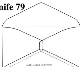
Mercantile Knife, side flaps with square side flap ends (20 mm); rough edges; made with Kenny rotary machine.
