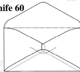
Middle West Envelope Co Knife, made with Smithe rotary machine, side flaps with square ends (15 mm), rough edges usual.
