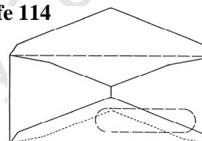
U.S. Envelope Co. Knife, side flaps with straight ends 28 to 30 mm. 110 x 241 mm.
