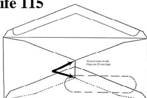
International Envelope Co. Knife, side flaps with straight ends 25 mm long. 110 x 241 mm.
