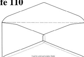
Mercantile Knife, rough edges; with square side flap ends (20 mm); made with the Kenny rotary machine. 105 x 241 mm.
