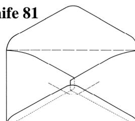
Middle West Envelope Co. Knife, side flaps with square side flap ends (15 mm), rough edges; made with Smithe rotary machine.
