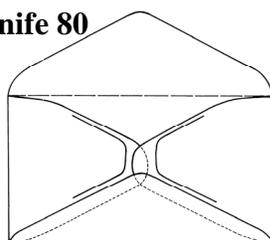
Mercantile Knife, made to match shape used on the Kenny rotary machines. Used for solid fronts, 1915-29; window fronts 1915-1949.
