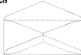
U.S. Envelope Company Knife, sharp corners on and bottom top flaps, 98 x 226 mm.
