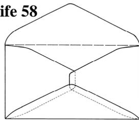
Mercantile Knife, made with Kenny rotary machines, side flaps with square ends (20 mm), rough edges usual.
