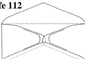
Middle West Envelope Co. Knife, intended to duplicate the shape of the Kenny rotary machine. 105 x 241 mm.
