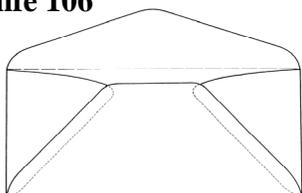
Plimpton & Morgan Knife & International Envelope Company, high back envelope, side flaps top curved with nearly circular tips (12 mm dia.), bottom flap is 95 mm tall. 105 x 241 mm.
