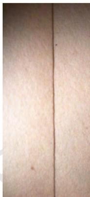
Envelope blanks cut with a knife from sheets (above) have straight edges and gradual curves, while rotary cut envelopes have rougher edges with nicks (below).
