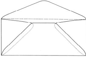
Plimpton Knife & U.S. Envelope Co Knife, used for window fronts after 1949, high back.
