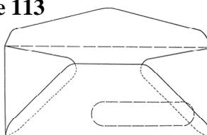
International Envelope Co. Knife, corners on top flap, high back (85 mm), compare to Knives 106 and 116, used for envelopes 3501A and 3501B only. 110 x 241 mm.
